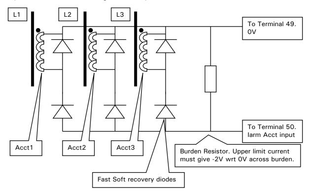
This circuit is required externally to generate an armature current signal. The Accts will typically be grain orientated silicon steel. This circuit is able to measure the current waveforms in the AC supply lines to the Stack. By combining the signal from each line through the diode bridge a representation of the armature current is generated across the burden resistor.
