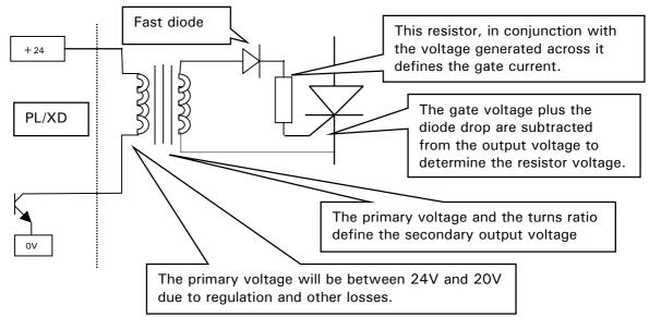
Example. The pulse transformer has a 2 : 1 ratio. The desired minimum gate firing current is 1 amp.
