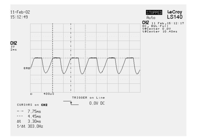
This is a discontinuous current waveform trace using Accts of diameter 150 mm, 4000 turns silicon iron grain orientated steel cores. Notice that there are no turn off tails normally associated with such cores. This is because they have been connected as described.
