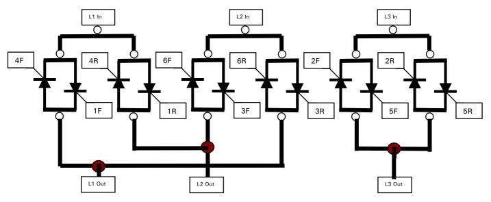
When 4 quadrant mode is selected the R pulses allow firing of a parallel bridge which introduces phase rotation at the output.
