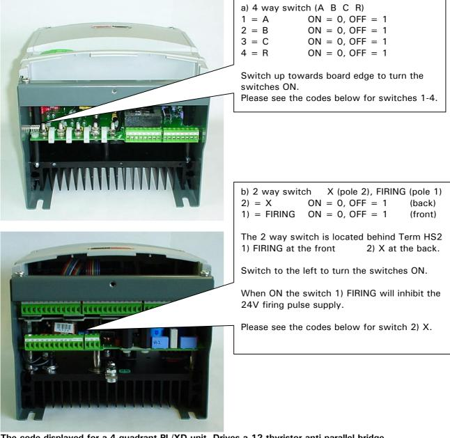
The code displayed for a 4 quadrant PL/XD unit. Drives a 12 thyristor anti parallel bridge.679)IDABCXRxxxMON(note ABC R are on 4 way switch, X is on 2 way switch)10111000Max Displayed Armature current3000.0 Amps. Max Displayed Field 32 Amps.
