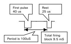
7.4.1 Field pulse transformer circuit (Voltage driven)
