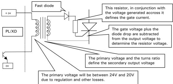
Example. The pulse transformer has a 2 : 1 ratio. The desired gate firing current is 0.32 amp.
