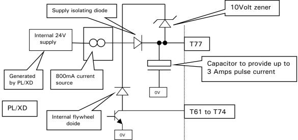
In the event of a short circuit the current source will limit the steady state short circuit current to a maximum of 800mA.
