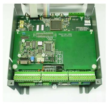
PROFIBUS card mounted on 'mounting board for profibus card' and fixed onto PL/X control card. Note. The front bar is removed from the PL/X here for picture clarity only.
