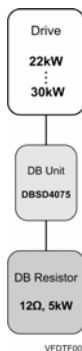
Figure 4.11 Combination of DB Unit – DB Resistor for drives with capacities of 22kW – 30kW
