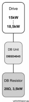
Figure 4.10 Combination of DB Unit – DB Resistor for drives with capacities of 15kW – 18,5kW
