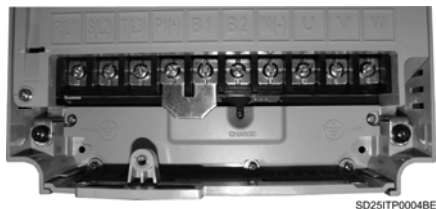
Figure 2.9 Power terminals detail. Frames 5 and 6
