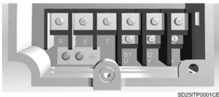
Figure 2.6 Power terminals detail. Frames 1 and 2
