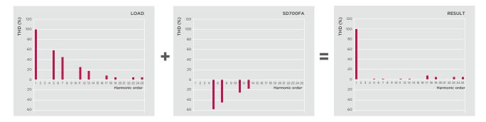
By setting the **full spectrum harmonic cancellation** the unit will not be focused on a specific harmonic number. Any harmonic content will be cancelled by injecting an opposite phase current wave form that results from subtracting the fundamental (50Hz) current wave.
