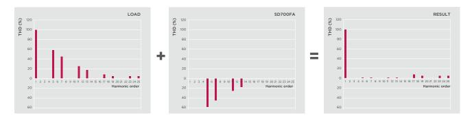
By setting the **full spectrum harmonic cancellation** the unit will not be focused on a specific harmonic number. Any harmonic content will be cancelled by injecting an opposite phase current wave form that results from subtracting the fundamental (50Hz) current wave.
