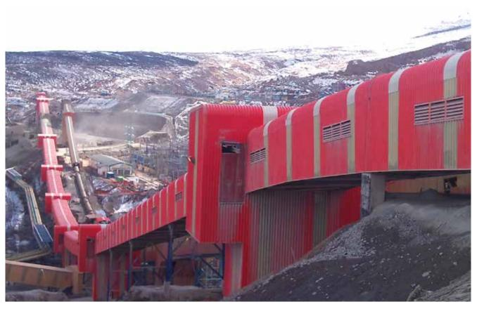
Downhill conveyor for high altitude mining.
