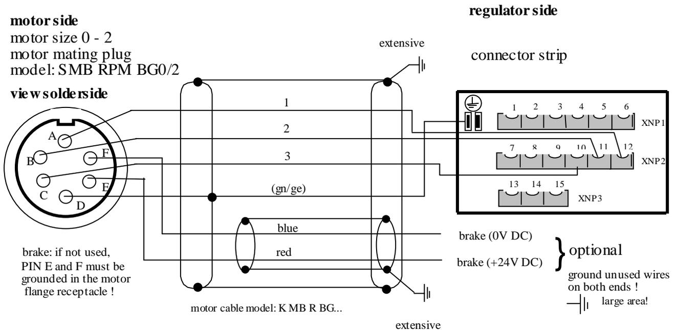
Motor-line-shield: on both ends, extensively connected!
