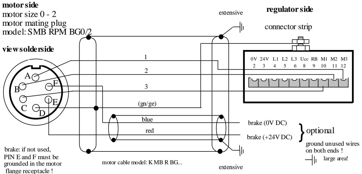
Motor-line-shield: on both ends, extensively connected!
