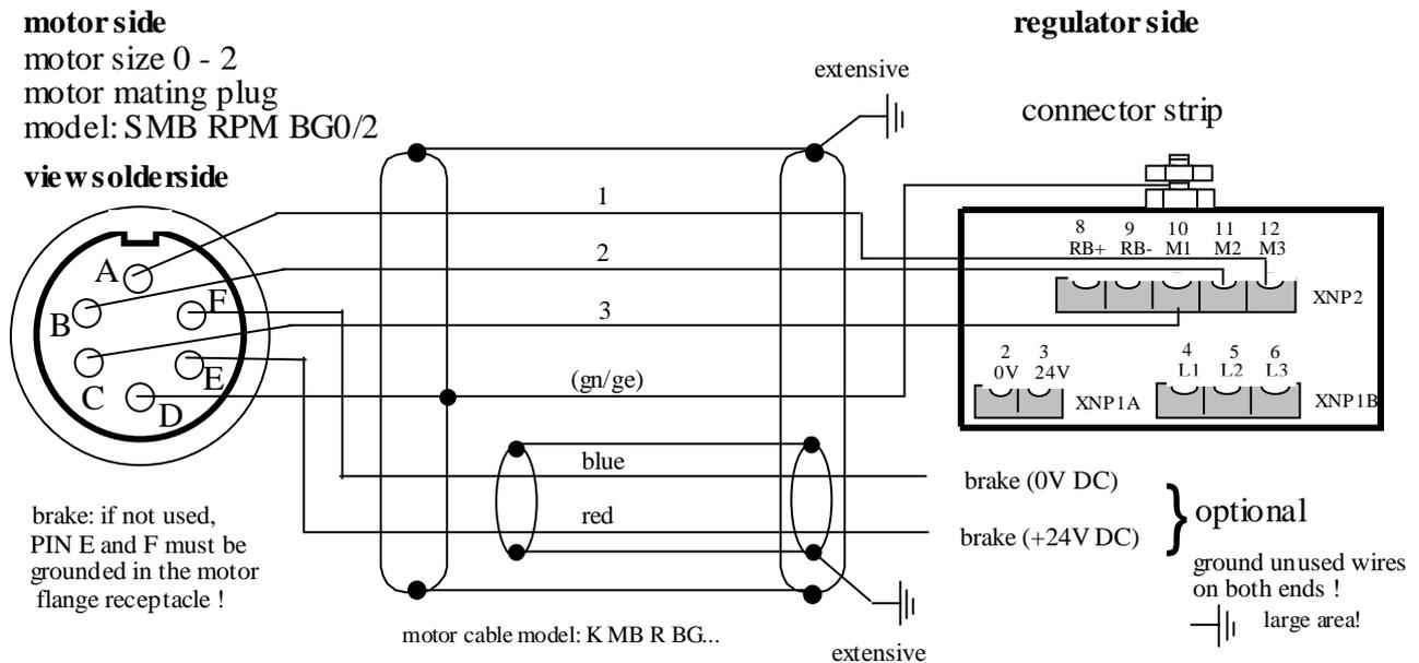
Motor-line-shield: on both ends, extensively connected!
