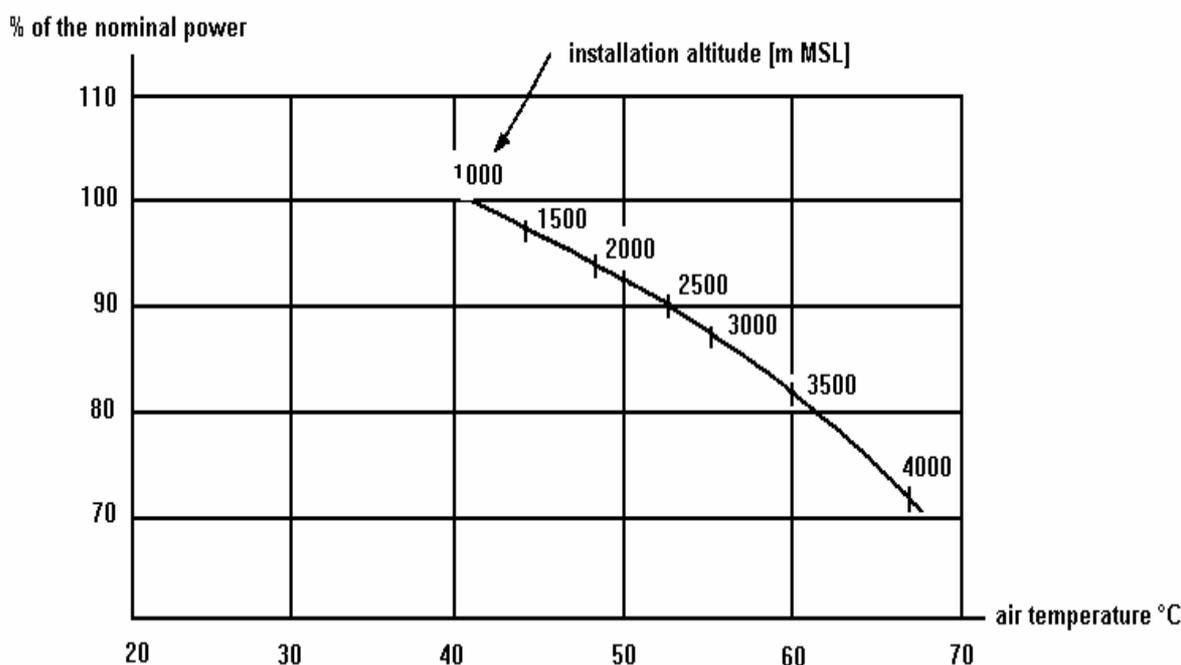
Check the air temperature and the installation altitude separately. Should there be different air temperatures and installation altitude at the same time, the factors for the permissible power must be multiplied.
