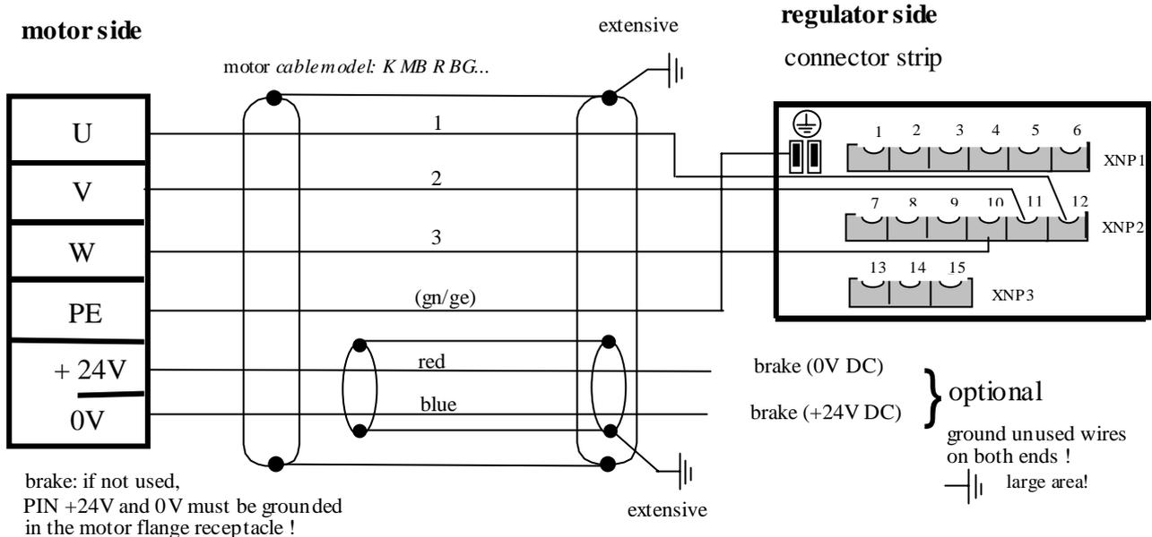
Motor-line-shield: on both ends, extensively connected!
