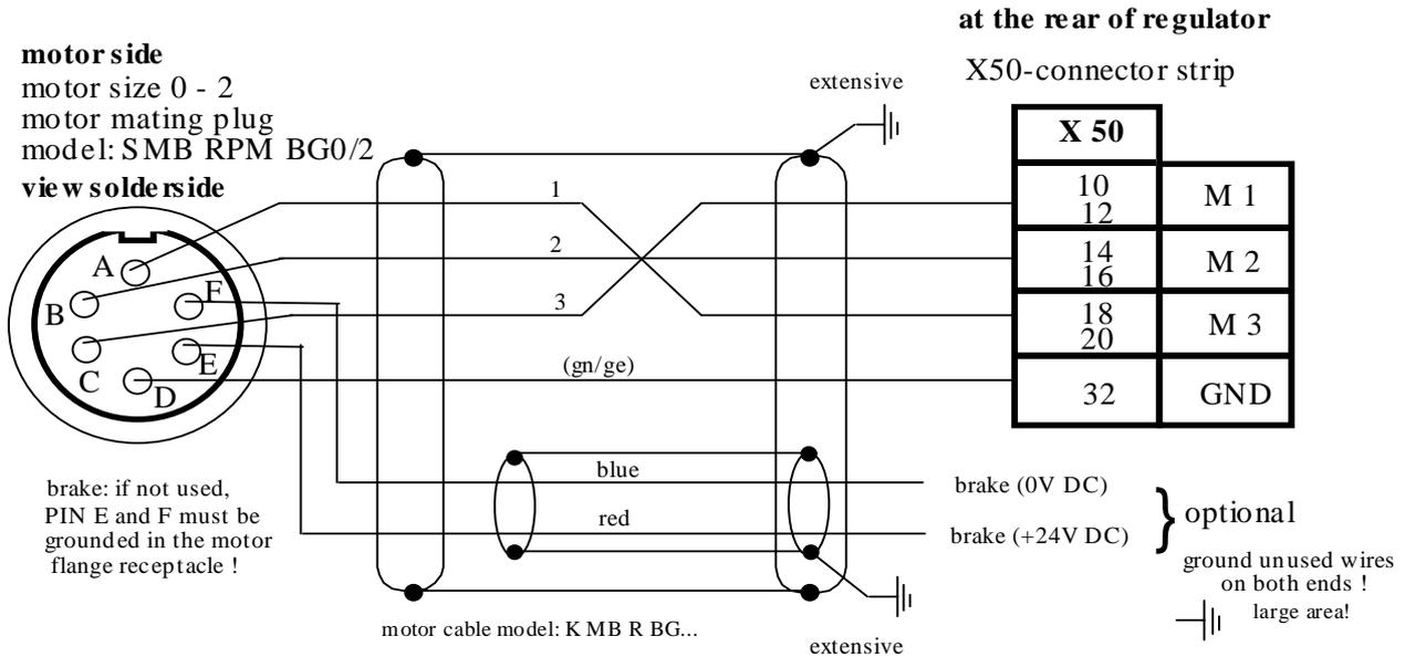
Motor-line-shield: on both ends, extensively connected!
