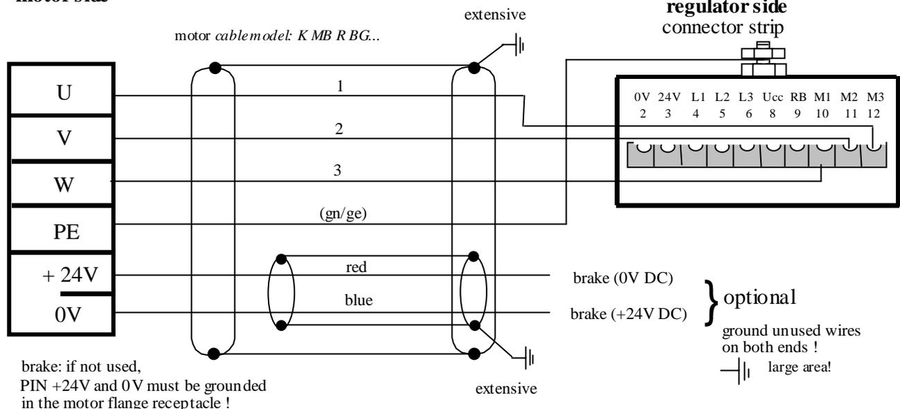
Motor-line-shield: on both ends, extensively connected!
