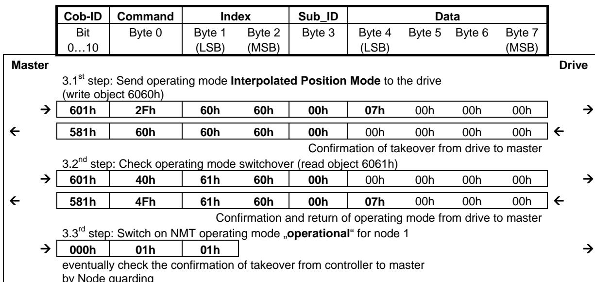
4. SYNC telegram and activation of the Interpolated Position Mode
