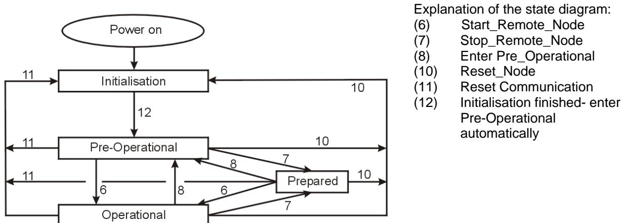
After power on the controller the CAN interface and the CAN services will be initialized corresponding to the Baud rate and the set node number.
