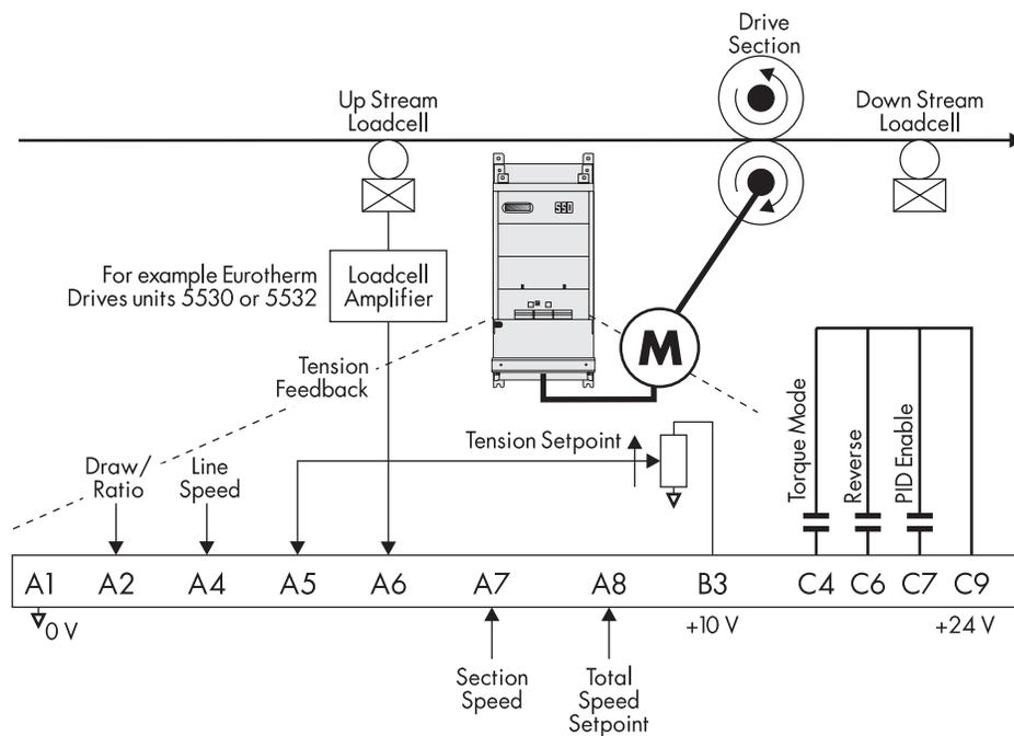
Figure 4.1 – Loadcell Application
