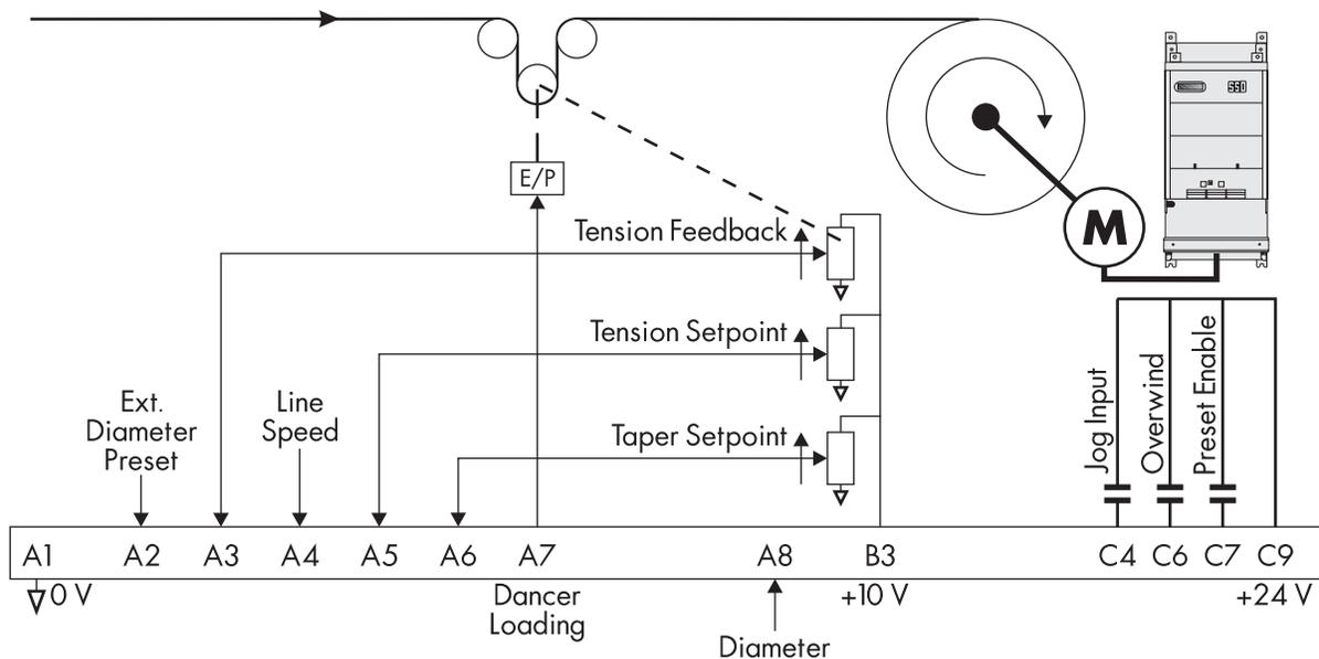
Figure 3.2 - Rewind SPW Application with Dancer Position Feedback
