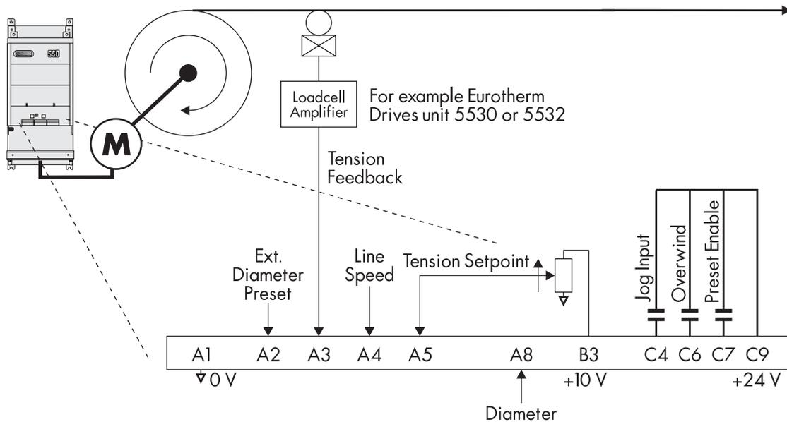
Figure 3.2 - Rewind SPW Application with Dancer Position Feedback
