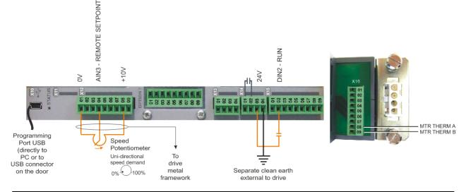
This is a basic connection diagram. For more detailed information on control connections, refer to Appendix B.
