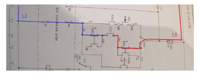
K237 in picture below, is old type synchronizer and in generator 1 you have the new FAS-113DQ component, same type as this one just modern. I can also see that the old K137 in generator 1 has broken before and replaced, the screw holes match the K237 in generator 2.
