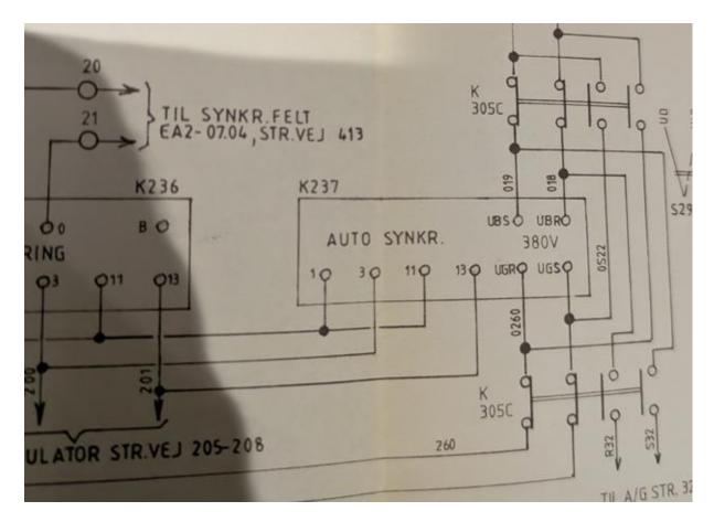
The only thing I can see is different between these two modules is that the new one requires a supply voltage. Use any 380V fuse inside the switchboard from generator 2 side, do not use busbar voltage to power component.
