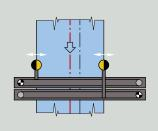
This support beam also features two carriages, each with its own independent drive unit. This means that the left and right sensors may be adjusted independently of one another. Due to a synchronous drive control, web offsetting is thus possible across the full width of the web.
