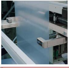
Ultrasonic sensor FX 4 on a rotary offset press
