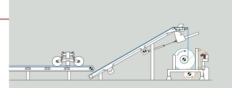
ELROLLER SRS 41 on a double-fold assembling line
