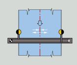
This version comprises two carriages, linked to one another via a toothed belt. The former are protracted or extended together via a drive unit.
